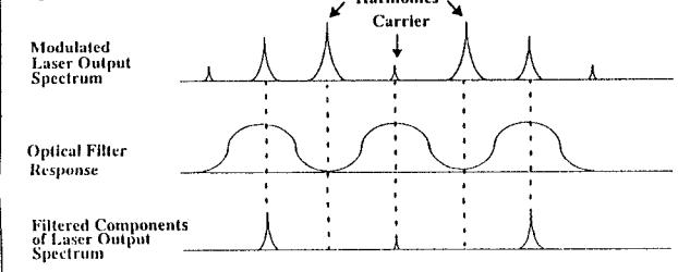
This filtering pattern also enables electronic stabilisation techniques to be employed in order to ensure that the laser wavelength remains locked to the peak of the filter pass band. In the experiment it was found that by housing the MZI in a polystyrene box the filter transmission peak remains relatively stable in relation to the laser wavelength. Once the desired harmonic components have been selected they are mixed on a high speed photodetector in order to generate the beat frequency.
