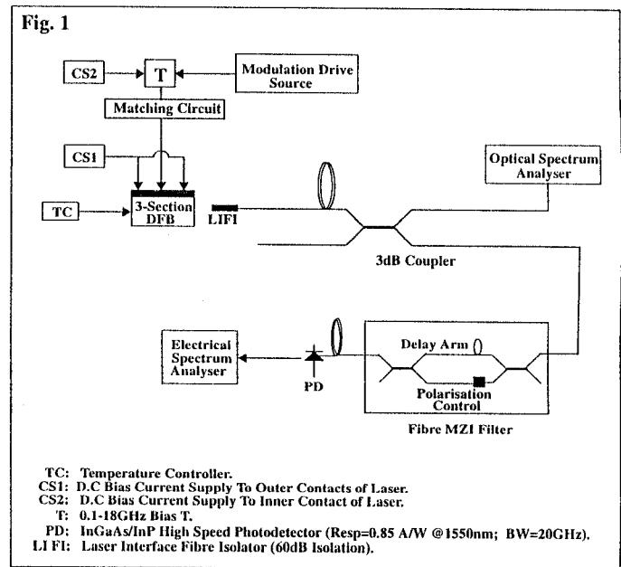
These components are selected using a Mach Zehnder interferometer (MZI) optical fibre filter in order to suppress unwanted harmonic components in the generated optical spectrum.
