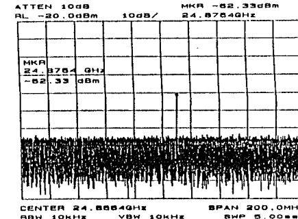
**Conclusion:** This technique produces microwave and millimetre-waves without the need for optical phase noise reduction techniques. Frequencies up to 25GHz have been generated with the potential to generate higher frequencies by filtering higher order harmonics.
